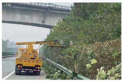
The hydraulic device is controlled via the multi-way solenoid valve by operating the control handle in the cab, so that the device could be lifted/lowered flexibly and retracted flexibly to implement the horizontal trimming, vertical trimming and trimming at varied height etc.
